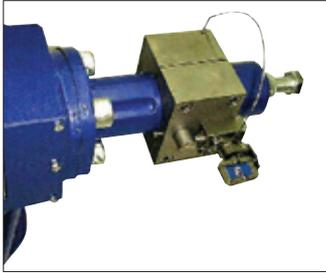
**Partial stroke test device (PSTD)**
