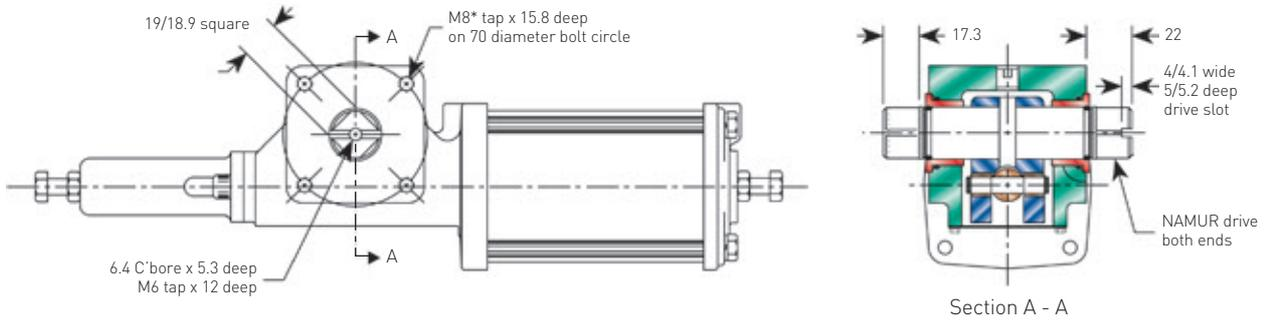
MODELS 023 THROUGH 100 - TOP AND BOTTOM OF HOUSING (SYMMETRICAL) ISO 5211-F12
