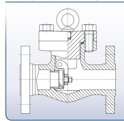
Small size swing check valves does not require lifting eyebolts as standard because of the low weight. Handling is normally performed on small valves by lifting with eye bolts or rods through flange holes. If required the bonnet design can be modified in order to include one screwed lifting eve bolts screwed on the top to facilitate valve installation into the piping system.
