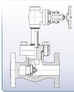
The removal of fluid in pipelines can be a frequent operation for some oil&gas industry applications. The drain/vent line can be added to the swing check design based on the customer requirements. Connections can be provided with permanent block valves, including plugs or blinds.
