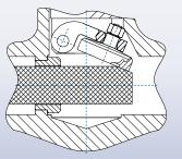
Swing check valves can be furnished with drain. Standard drain connections consist of a drilled, tapped, and plugged hole at the ASME B16.34 "G" location. Other types of drains, including welding, or threaded nipples, can also be furnished when specified.
