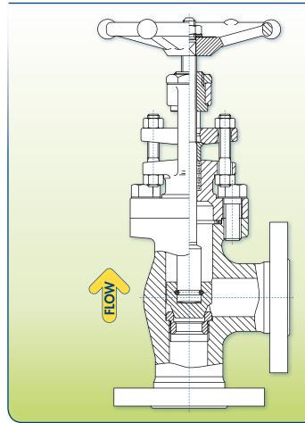
The Angle pattern globe valve is a modified version of "T"-Pattern Globe valve with inlet and outlet at right angles. When fitted at a change in piping direction, this valve eliminates a bend and has the advantage of smaller pressure drop than a conventional "T" pattern globe valve.
