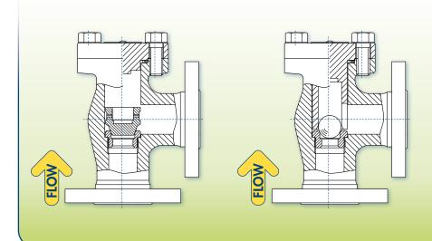
The Angle pattern check valve is a modified version of a standard check valve with inlet and outlet at right angles. When fitted at a change in piping direction, this valve eliminates a bend and has the advantage of smaller pressure drop than a conventional check valve.
