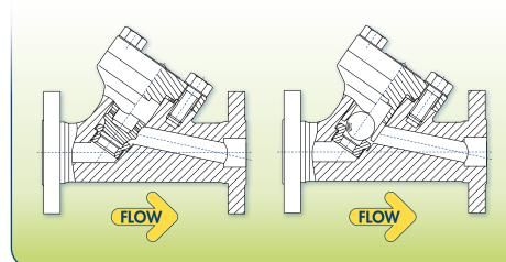
The "Y"-Pattern check valve is a modified version of a standard check valve.
