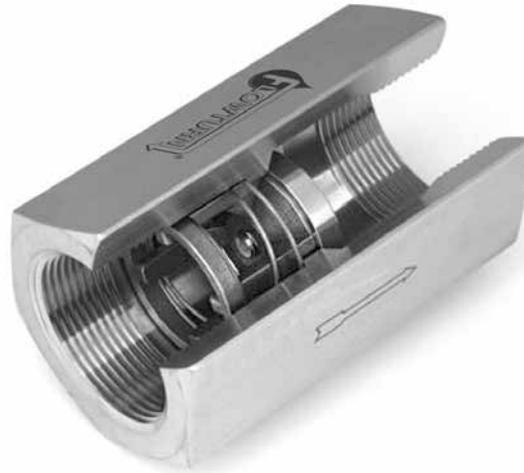
The CAV-3 check valve is a one piece body machined from bar stock and is designed for minimum pressure drop. The valve has a light weight compact design that provides maintenance-free dependable service. 10,000PSI Model also available to 2"
