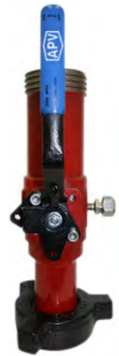
Ball Valve c/w Integral Hammer Union Ends for Quick Changeouts on Tanker Unloading Manifolds.
